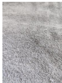
Figure 7: Leather flesh side before skiving machine
