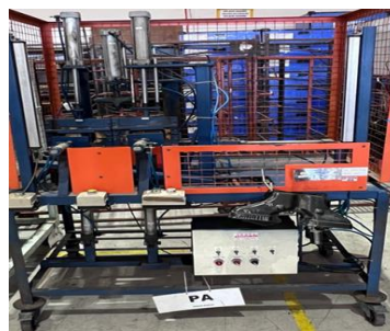
Figure 4.2: New Punching jigs machine
