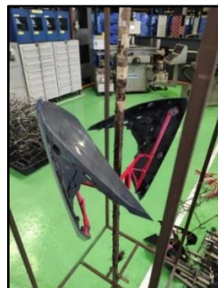
Figure 3.1: Current sub hanger of Mole 1
