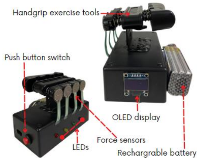
Figure 5: Electronic handgrip rehabilitation exercise force measuring by using force sensor
