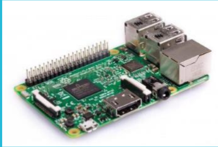
Fig. 2.0: A Raspberry PI 3 Controller
