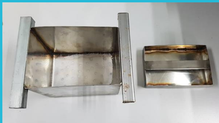
Figure 2: Part for extracting coconut milk
